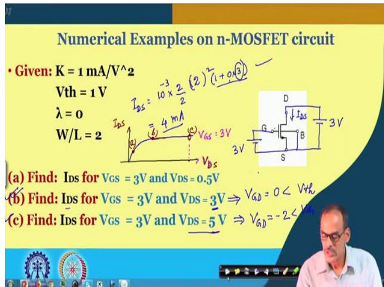
Now, let us look into the next part-(b) so here  $V_{GS}$  we are keeping same, but then  $V_{DS}$  we are changing to 3 V. So, what we have here it is to consider this part we do have 3 V here, body is connected with this and then we do have here also we do have 3 V. So, as you can see here  $V_{GS}$  is more than  $V_{th}$  of course, the device is on and however  $V_{DS}$  since it is equal to  $V_{GS}$ . So, drop across this one it is just 0 voltage.
