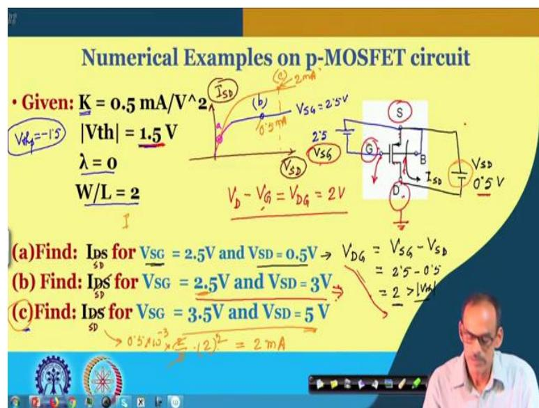
It is similar but of course, I have changed the parameter. So, what are the changes we do have here, the  $V_{th}$ ,  $|V_{th}|$  it is instead of 1 we are considering 1.5. In fact, you may recall  $V_{thp}$  sometimes if it is given directly it may be given this  $V_{thp}$  is  $-1.5$  ok, it is I should say it is same.
